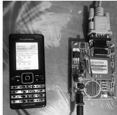
Fig. 4. Sending SMS report of parameters – Simulation result using Proteus.
